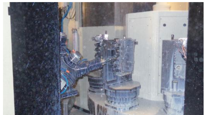
300 V – Wide axes travels allow to work most of the large size car engine components
