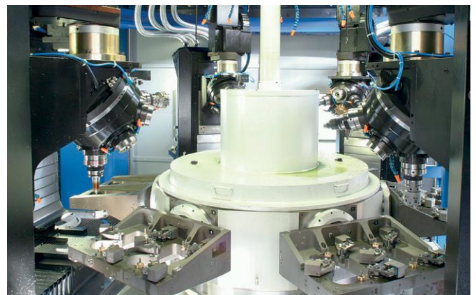
300 H – internal view showing a typical configuration with revolver head modules and a special application as regards the clamping fixtures
