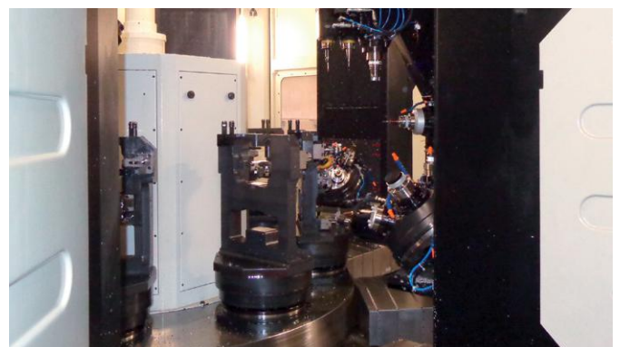
300 V – Engineered machining heads, horizontal six spindles turret and vertical single/twin spindle heads which are assembled on the same module
