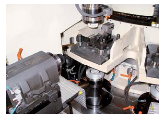
IMASTRANSFER – Up to three modules simultaneously working along orthogonal directions with large use of CNC axes.
